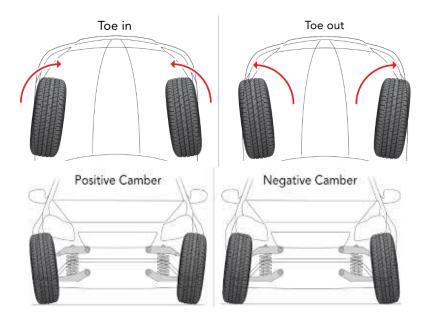
Checking the wheel alignment of your vehicle regularly can save you money by prolonging the life of your tyres by up to 12,000 miles and improving fuel efficiency.
